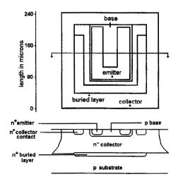
Fig. 3. Schematic layout and cross-section of the transistor.
