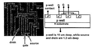
Fig. 1. Optical micrograph of the n-channel transistor. The diagram below represents the available contacts.
