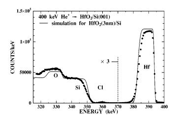
FIG. 1. High-resolution RBS spectrum of  $HfO_2/Si(001)$  observed at a scattering angle of 50°. The incident ion is 400 keV He<sup>+</sup> and the incident angle is 50.24°. The solid curve shows a simulated spectrum for  $HfO_2$  (3 nm)/Si(001).
