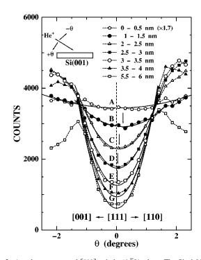
FIG. 3. Angular scan around [111] axis in  $(1\bar{1}0)$  plane. The Si yields for different depth regions of 0.5 nm wide are shown as a function of the angle of incidence around the [111] channeling direction. The depth shown is measured from the HfO<sub>2</sub>/SiO<sub>x</sub> interface. The channeling dip shifts towards larger incident angle with decreasing depth.
