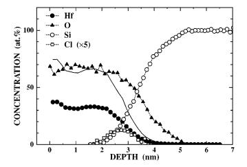
FIG. 2. Elemental depth profiles for Hf, Si, O, and Cl ( $\times$ 5) in HfO<sub>2</sub>/Si(001). The solid curve shows twice the Hf concentration. There are excess oxygen atoms in the interface region, showing formation of a thin SiO<sub>x</sub> layer between the almost stoichiometric HfO<sub>2</sub> film and Si substrate.
