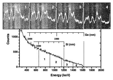
Fig. 3. 100  $\mu$ m × 100  $\mu$ m CCM maps of the same spatial location, generated from four energy windows with sample BF1040 rotated +0.2° off axial about the [011] direction. The intensity profiles across the horizontal direction for each map are given.
