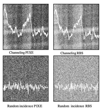
Fig. 4. 100  $\mu$ m × 100  $\mu$ m channeling and random incidence PIXE and RBS maps of sample BF1040. The intensity profiles across the horizontal direction for each map are given.
