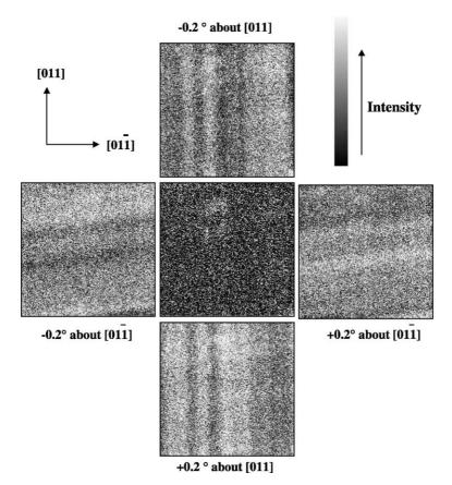
Fig. 2. 100  $\mu$ m × 100  $\mu$ m CCM maps of sample BF1040 for  $\pm 0.2^{\circ}$  rotation off axial about [011] and [011].
