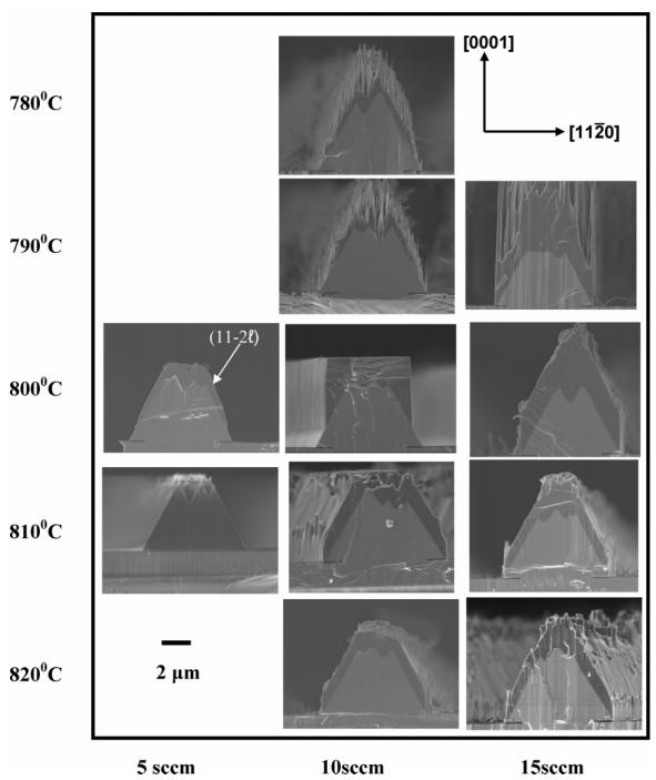
Figure 1. Morphological changes in ZnO grown on the FACELO GaN templates with different growth temperature and oxygen flow rate. Growth time was 0.5 h.
