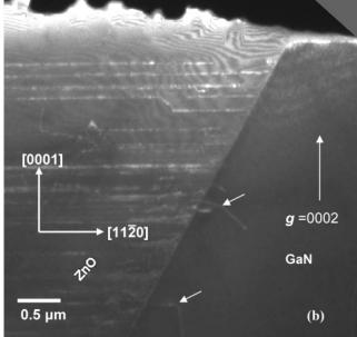
**Figure 2.** (a) HRTEM image and the corresponding SAED pattern of ZnO/FACELO GaN interface grown at 800 °C with the oxygen flow rate 10 sccm. (b) Cross-sectional TEM image with g=0002 near the interface of ZnO/FACELO GaN grown at 800 °C with the oxygen flow rate 10 sccm.
