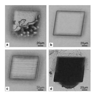
Fig. 3. Proton irradiated samples (a) underexposed sample, partially removed, (b) correct exposure, collectively removed area with smooth bottom, (c) overexposed sample, uneven bottom, (d) overexposed sample, melted area, droplet melted.
