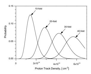
Fig. 1. Probabilities of multiple proton latent track overlap as a function of track density. The diameter of a single latent proton track was assumed to be 3 nm.
