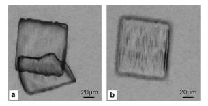
Fig. 4. Alpha irradiated sample (a) after 5 s etching (Note: the "lid" is visible here, the bottom side of it is already out of focus, i.e. it is raised off the surface.) (b) after 10 s etching (the lid is gone, only the removed pit is visible).
