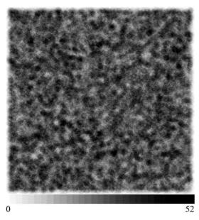
Fig. 2. Grayscale plot (white: minimum intensity, black: maximum intensity) of the multiple latent track overlap based on our Monte Carlo calculations. The square represents  $100 \times 100 \text{ nm}^2$  beam spotsize, and a single proton track diameter was 3 nm. The total number of protons was  $3.75 \times 10^4$  on this surface  $(3.75 \times 10^{18} \text{ m}^{-2})$ .
