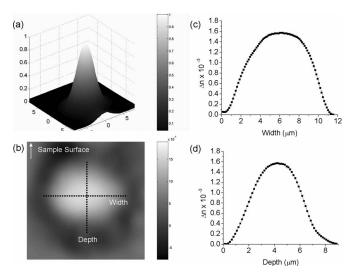
FIG. 2. (a) Near-field mode profile measured from the waveguide fabricated with the highest fluence  $(1\times10^{16} \, \mathrm{protons/cm^2})$ . (b) Recovered two-dimensional 2D refractive index profile and line profiles through the center of the mode along the (c) width and (d) depth of the sample.
