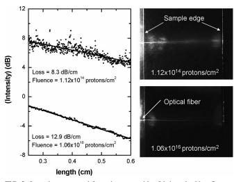
FIG. 3. Loss data measured from the waveguides fabricated with a fluence of  $1 \times 10^{14}$  protons/cm<sup>2</sup> and  $1 \times 10^{16}$  protons/cm<sup>2</sup>. The loss values we obtained ranged from 8.3 to 12.9 dB/cm.
