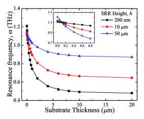
FIG. 2. (Color online) Variation in the simulated LC resonance frequency  $(\omega)$  as the substrate thickness is increased for SRRs of height 200 nm (black curve, squares), 10  $\mu$ m (red curve, circles), and 50  $\mu$ m (blue curve, triangles). The inset shows details of the region where the substrate is vanishingly thin, and reveals that the three curves cross.
