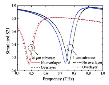
FIG. 3. (Color online) Effect of substrate thickness on sensitivity: shift in  $\omega$ upon addition of 1  $\mu$ m overlayer of  $\epsilon$ =2 onto SRRs on silicon substrates 1  $\mu$ m thick and 70  $\mu$ m thick.
