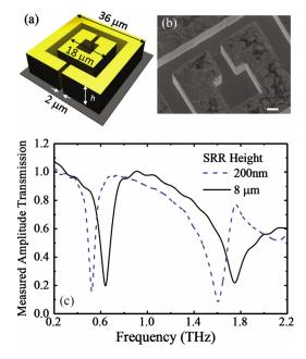
FIG. 1. (Color online) (a) Schematic diagram of a SRR illustrating the dimensions used in this study and the SRR height parameter (h), (b) electron micrograph of high aspect ratio SRR with h=8  $\mu m$  (scale bar=2  $\mu m$ ), and (c) measured THz spectra for SRRs of different heights.
