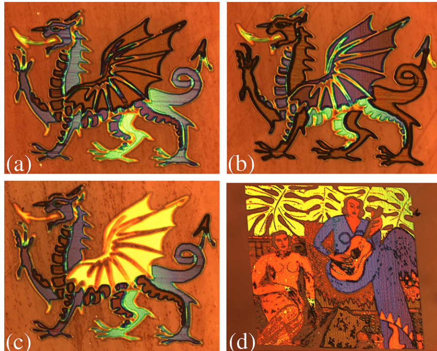
Fig. 4. (a)–(c) Reflection images of 400 \times 400 \mu\text{m}^2 regions irradiated with different overlaid scan patterns, corresponding to different doses to form dragon images. (d) Reflection image of miniature version of ‘La Musique’ painting (Henri Matisse) which was created by irradiating a 500 \times 500 \mu\text{m}^2 area with different doses ranging from 4 \times 10^{14} to 1.5 \times 10^{15}/\text{cm}^2 . In all cases the sample was illuminated with white light.
