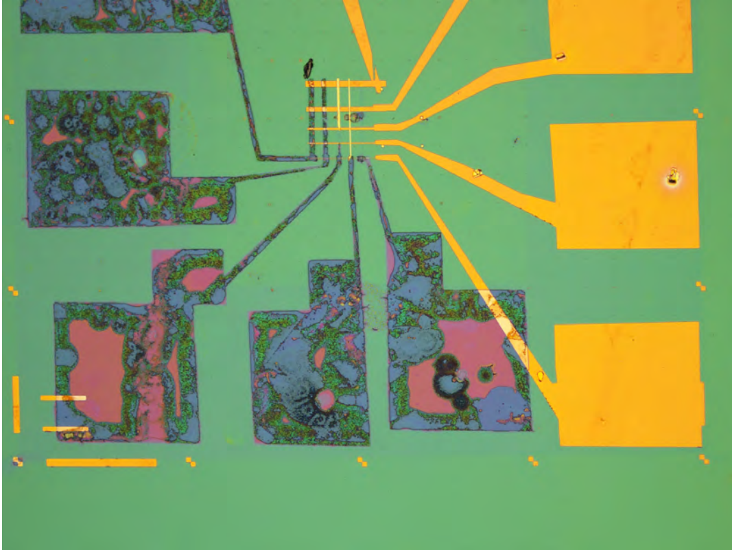
Figure 11: The local top gate patterns ruined by hot acetone ( T = 60^{\circ}\text{C} ). The hot acetone appears to partially dissolve the e-beam exposed LOR while leaving the unexposed and the laser exposed LOR in tact.
