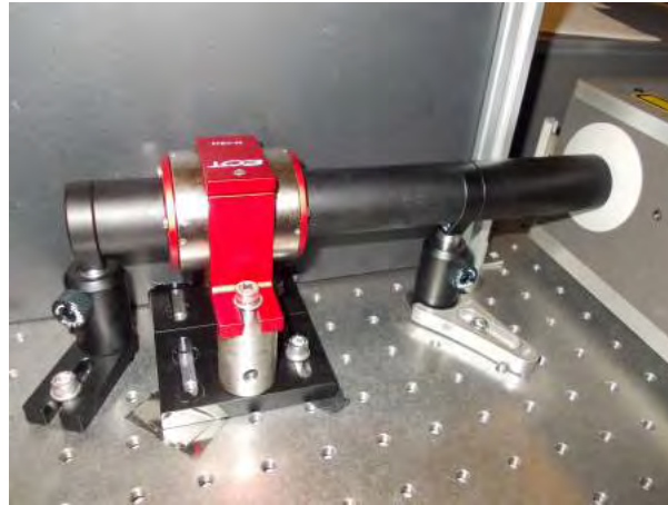
Figure 5.2: Mounted optical isolator, with safety tubes to house the high power beam.
