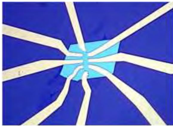
Figure 4.5: A typical 8-probes device with Hall bar geometry.
