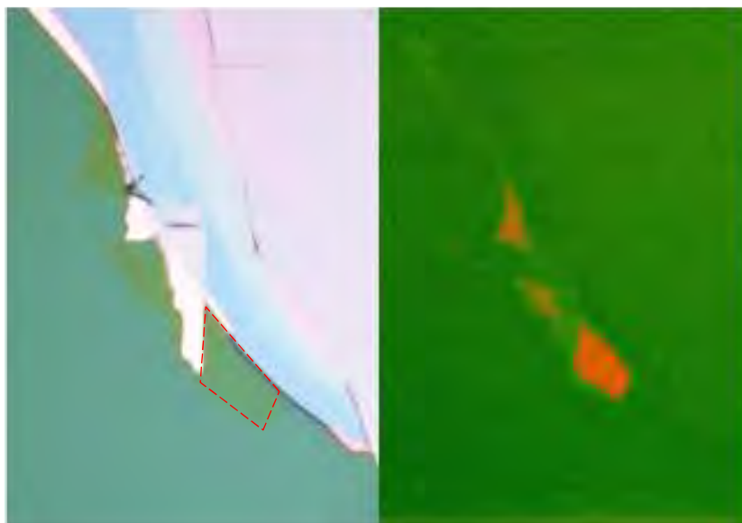
Figure 1.7: Photoluminescence effect. Red dotted lines indicate the monolayer MoS 2 . Photos are taken by Nikon Eclipse LV100DA, epi-Fluorescent Microscopy 2 with external mercury lamp source and 10s exposure.
