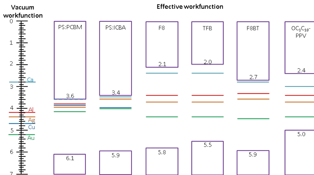
Figure 17: Energy level diagram for PS:PCBM(1:3), PS:ICBA(1:3), F8, TFB, F8BT and OC 1 C 10 -PPV devices with different metal electrodes
