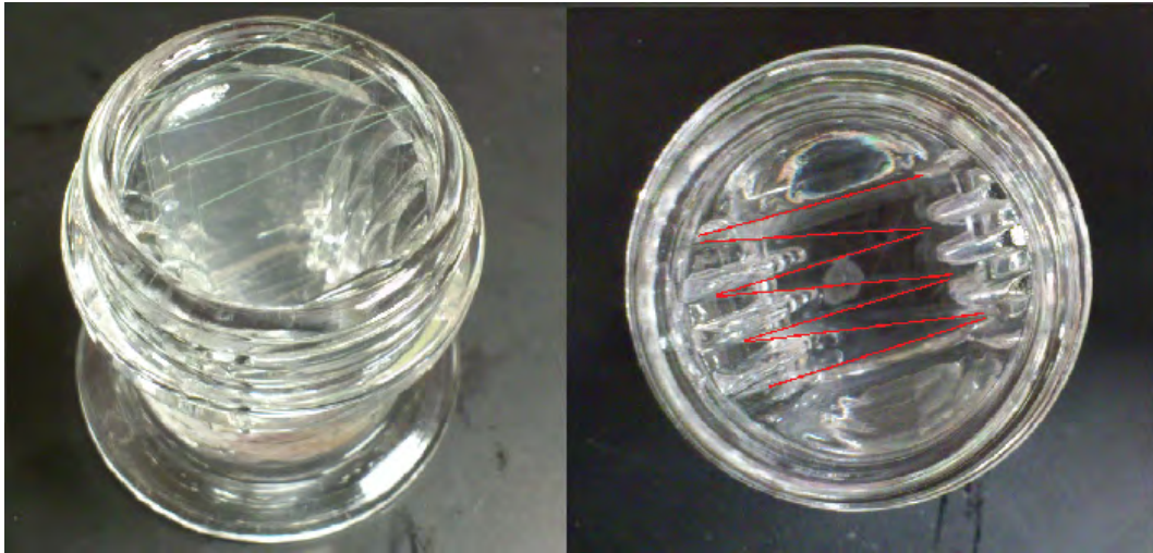
Figure 3.4: Views of the glass surfaces inside the jar, and the zig zag pattern of the glass shown in red lines
