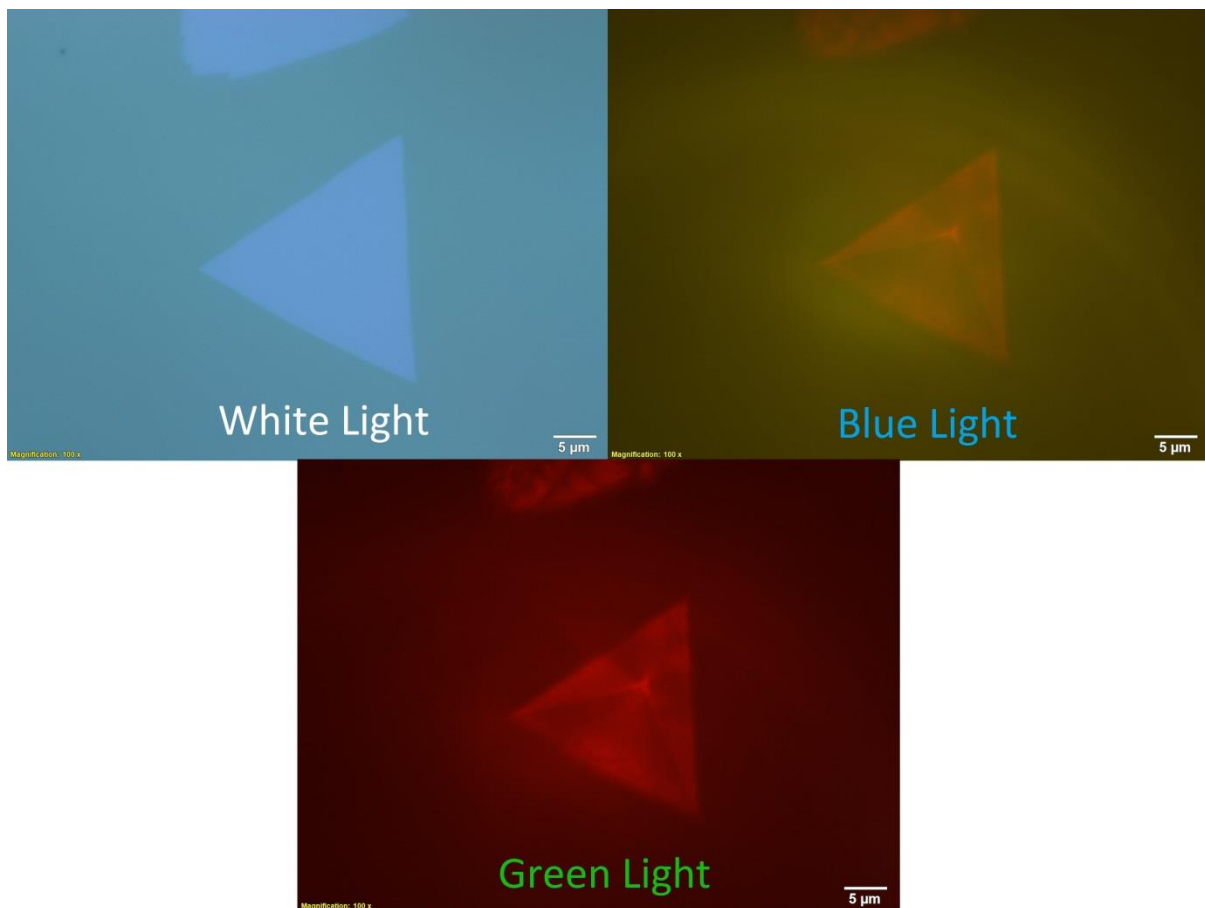
Fig 36: Fluorescence Microscopy results for WS 2 flake on Sapphire
