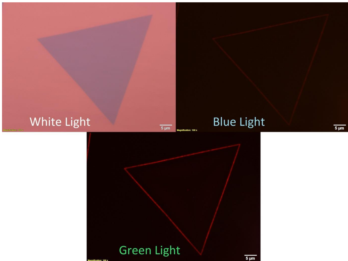
Fig 37: Fluorescence Microscopy results for \text{WS}_2 flake on \text{SiO}_2/\text{Si}
