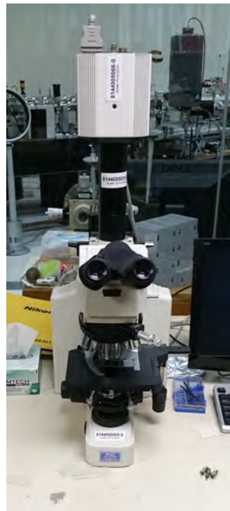
Figure 4.5: Optical Microscope Used for Measurement - Varying magnifying lens could be switched to view at higher magnifications.
