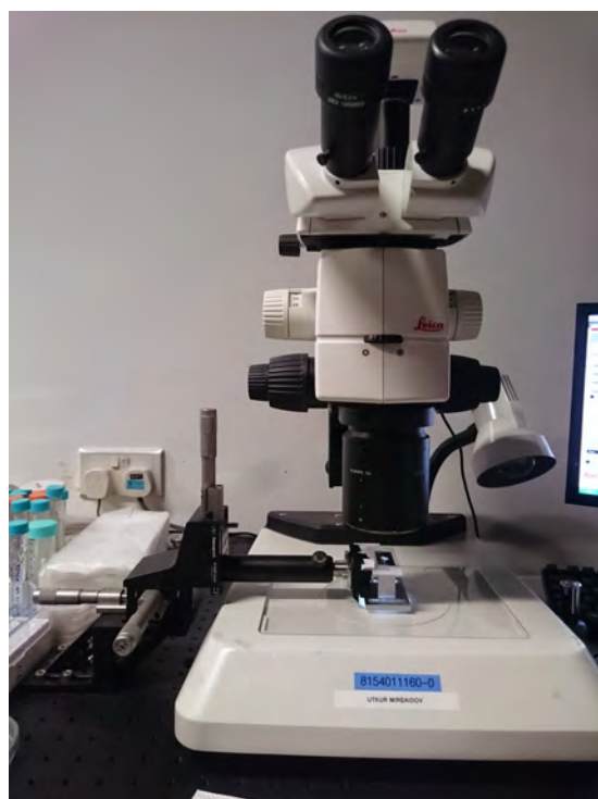
Figure 4.4: Light Microscope Used for Alignment - The top piece of the double aperture sticks onto a glass slide with aid of tiny droplets of water and secured to a 3-axis movable stage. The bottom piece also sticks to the glass slide with water but it is placed on a stationary stage. Using the microscope to look through the window, the top piece is slowly maneuvered in the x- and y-direction over the bottom piece till the double aperture aligns before it is lowered and glued.
