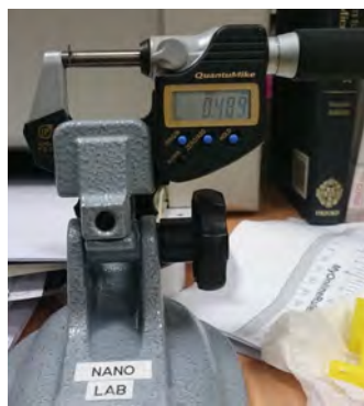
Figure 5.18: Micrometer Screw Gauge used to measure the thickness of wafer
