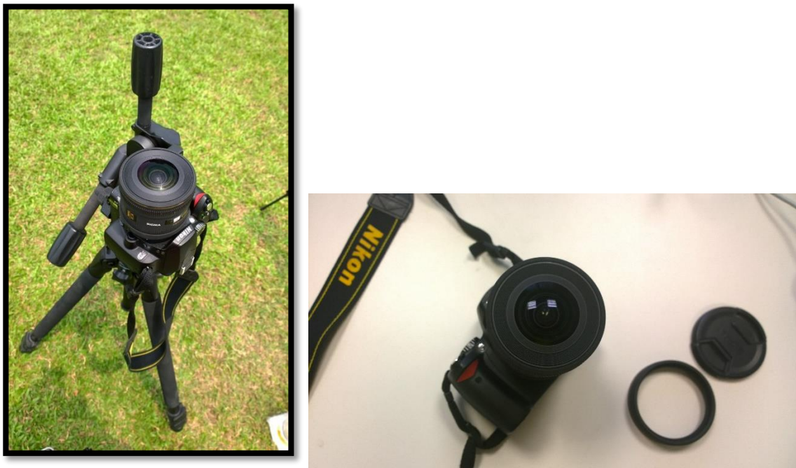
Figure 12 Nikon D60 4.5mm EX Sigma Fish-eye lens with 180 ° angle of view
