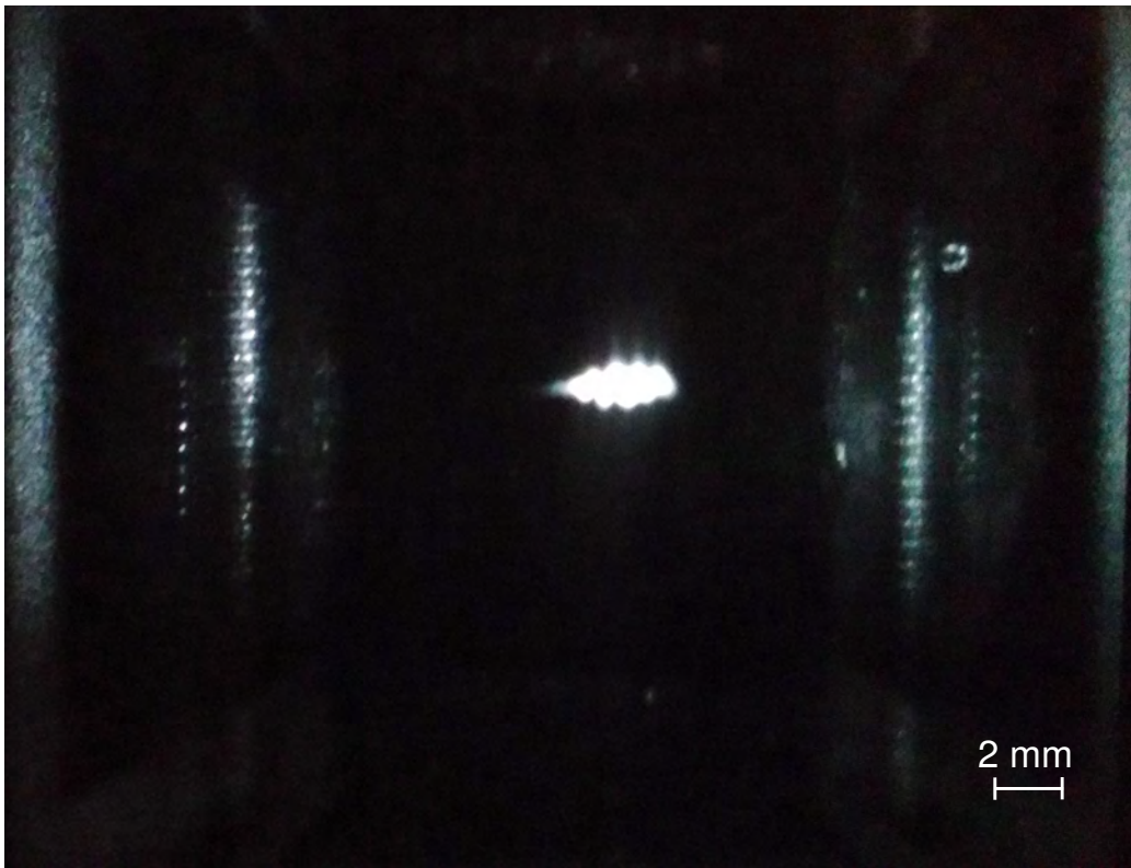
Figure 3.1: The picture of the elongated cloud of cold ^{87}\text{Rb} . For this cloud, we set the red detuning of the cooling laser as 10 MHz. The coil current was around 2.5 A, while the power on each MOT beams (around 1 inch in diameter) is around 20 mW.
