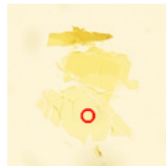
Figure 21 Optical images of bilayer MoS 2 using Koehler illumination under high light intensity.
