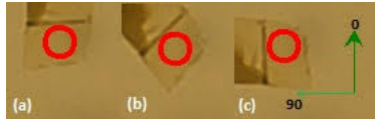
Figure 60 Optical image of bP crystal of 2.87 nm thickness with graphene encapsulation placed at (a) 0°, (b) 45°, and (c) 90° with respect to a polarizer whose direction is labeled with the green arrow on the left.
