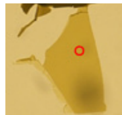
Figure 14 The red circle in the figure shows the detection area of the spectrometer, placed on a \text{MoS}_2 sample.
