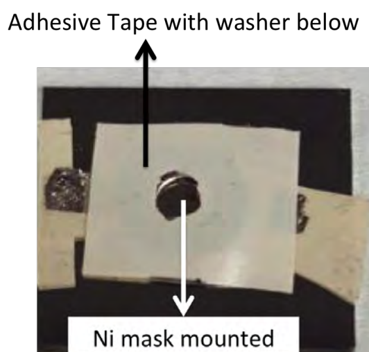
Figure 4.5: Mask Mounting Method 4 - MMM3 but with added tapes below to help adjust the tension on the Ni mask even after the mask has been mounted onto SS.
