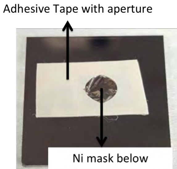
Figure 4.3: Mask Mounting Method 2 - First cutting a tiny aperture in adhesive tape before a strip of Ni mask is stretched across the aperture pasted down onto the sticky side of the tape. The entire tape is then stretched and pasted onto SS
